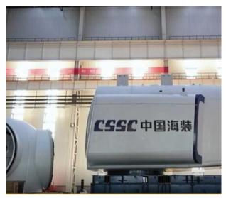
The rotor hub and nacelle of a new 18-MW offshore wind turbine from a subsidiary of China State Shipbuilding Corp. is shown at its factory. Source: CSSC Haizhuang
